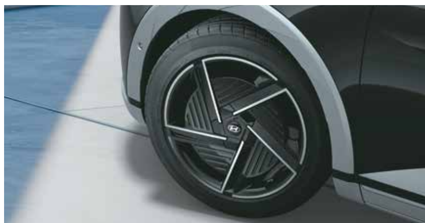
R20 (D=512.8 mm) Aero alloy wheels
