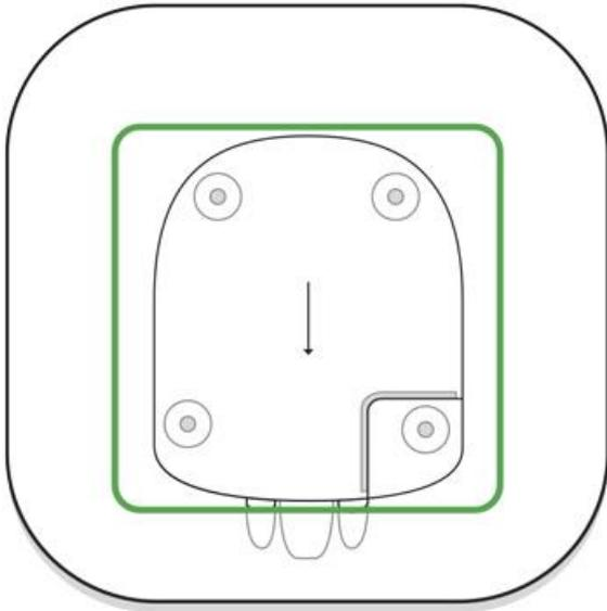
Be careful and do not damage the tamper protecting the hub from dismantling!
