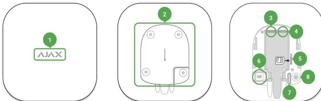
2. Smart Bracket attachment panel (perforated part is required for actuating the tamper in case of any attempt to dismantle the hub)
