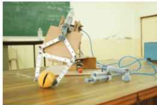
Hydraulic Robot: Robotic arm with three dimensional movement.
