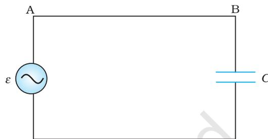
FIGURE 7.8 An ac source connected to a capacitor.
