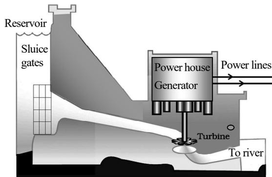
In order to produce hydel electricity, high-rise dams are constructed on the river to obstruct the flow of water and thereby collect water in larger reservoirs. The water level rises and in this process the kinetic energy of flowing water gets transformed into potential energy. The water from the high level in the dam is carried through pipes, to the turbine, at the bottom of the dam .
