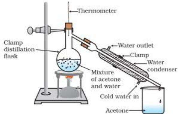
*Separation of two miscible liquids by distillation*
