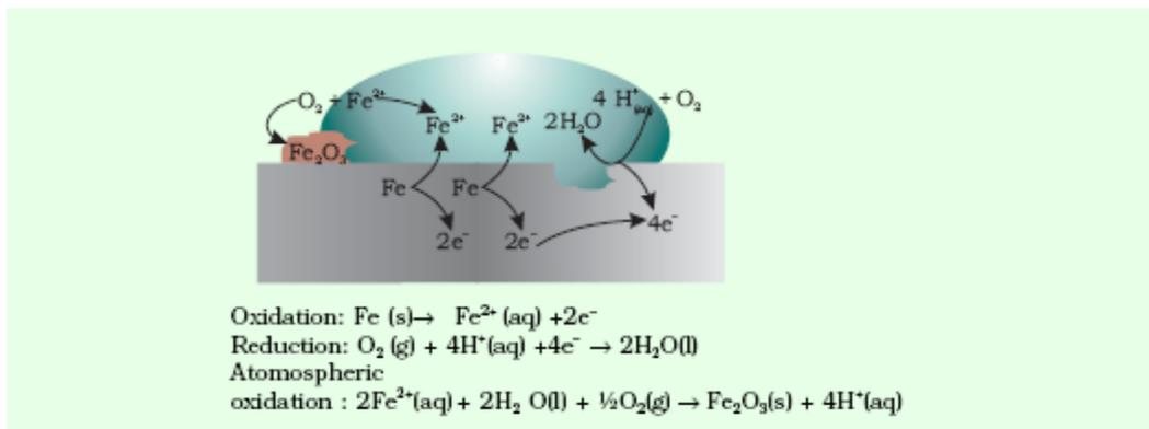
Fig. 5.14 Corrosion of iron in atmosphere.
