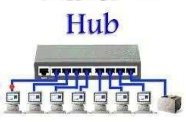
3. **Switch** :- A switch is a network device which is used to interconnect computers or devices on a network. It filters and forwards data packets across a network. The main difference between hub and switch is that hub replicates what it receives on one port onto all the other ports while switch keeps a record of the MAC addresses of the devices attached to it and forwards data packets onto the ports for which it is addressed across a network, **that's why switch is intelligent Hub.**
