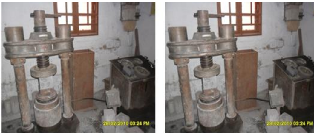
Figure 10: Compressive Strength Test Being Conducted
