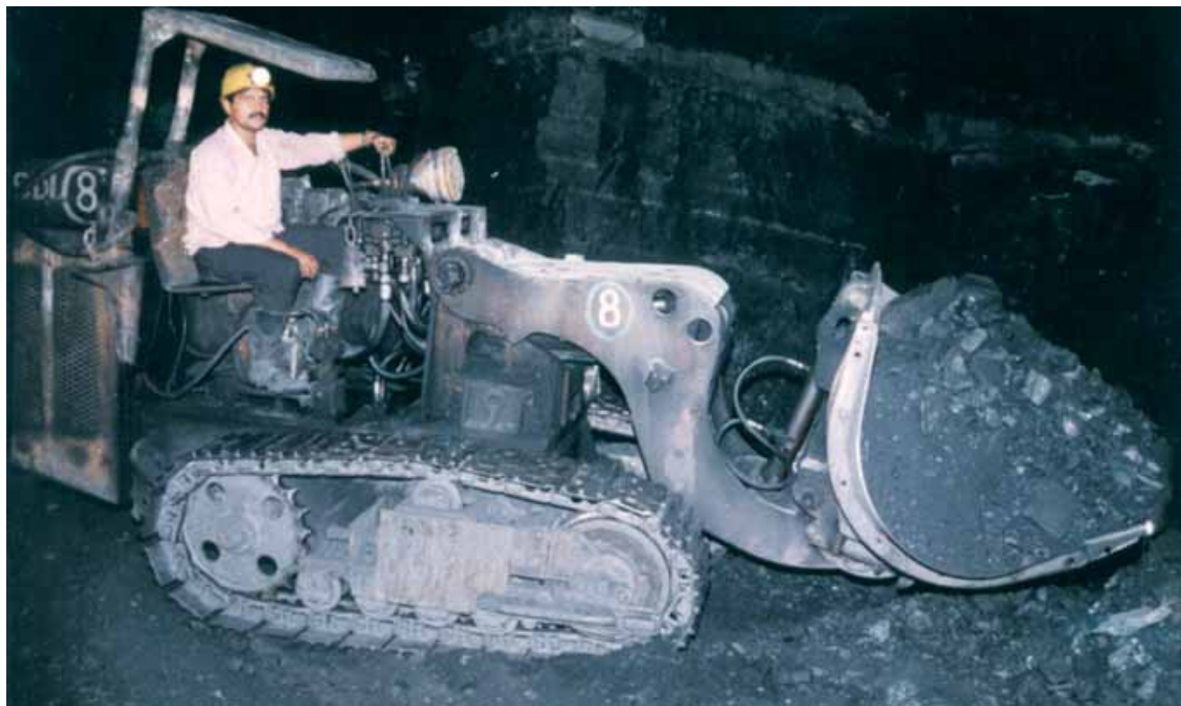
Side Discharge Loader - a machine works in Under Ground Coal Mine for loading coal in small locomotives
