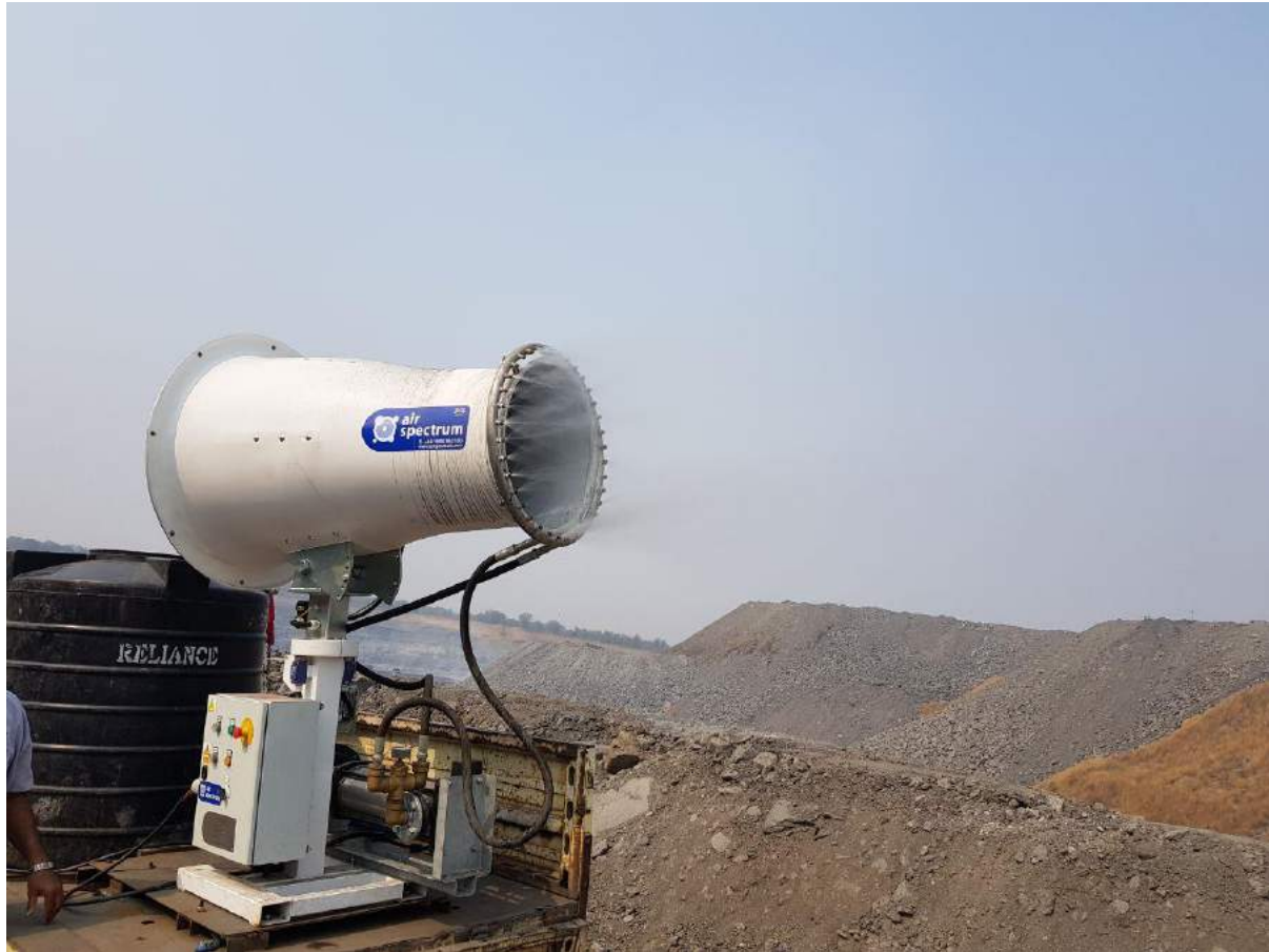
Fig. 30-Dust Controlling Arrangement in CIL Mine
