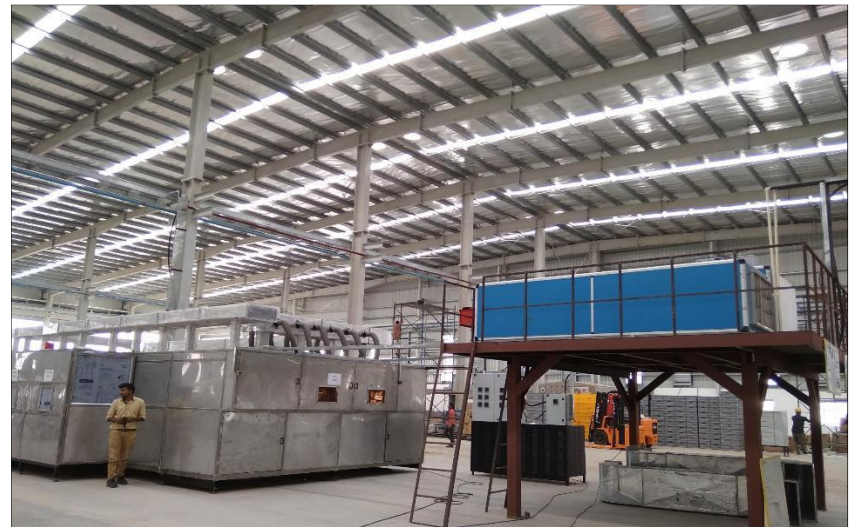
Surface treatment-hard coat installation
